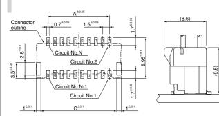
Note: 1. The above figure is the figure viewed from the connector mounting side. 2. Tolerances are non-cumulative: ±0.05mm for all centers.
