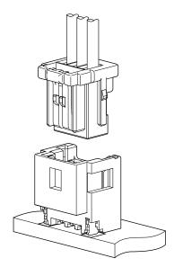
While realizing the space saving, this is the connector having the secure lock structure. By this, it is prevented the housing coming off by handling the wires or adding the vibration. This connector is very small, and it is possible to suppress the inverted insertion and achieves a clear insertion feeling.
