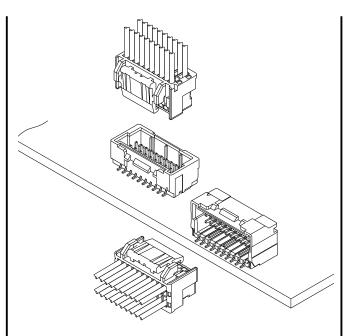
In 1.0 mm pitch and dual-row secure lock type connector, this NSHD connector realizes a top grade of a space saving in the industry and supports a high densification of equipment.
