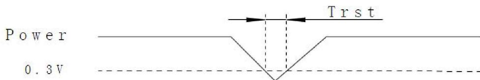
Figure 3-8 Power Cycle requirement
