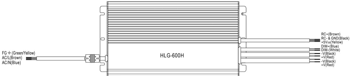
※ Built-in 3 in 1 dimming function, IP67 rated. Output constant current level can be adjusted through output cable by connecting a resistance or 0 ~ 10Vdc or 10V PWM signal between DIM+ and DIM-.
