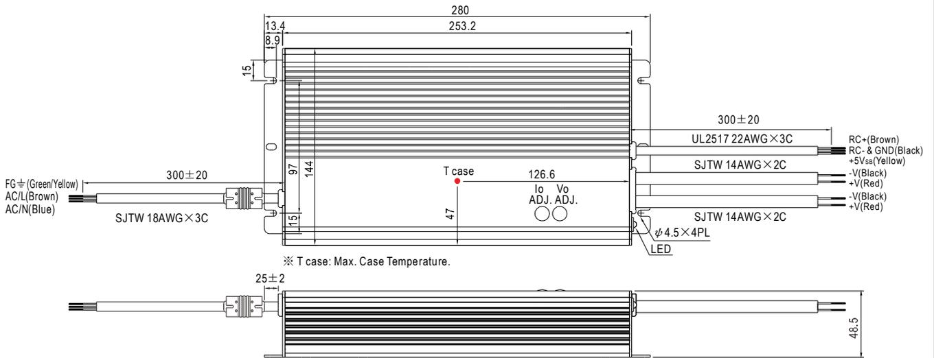
※ IP65 rated. Output voltage and constant current level can be adjusted through internal potentiometer.
