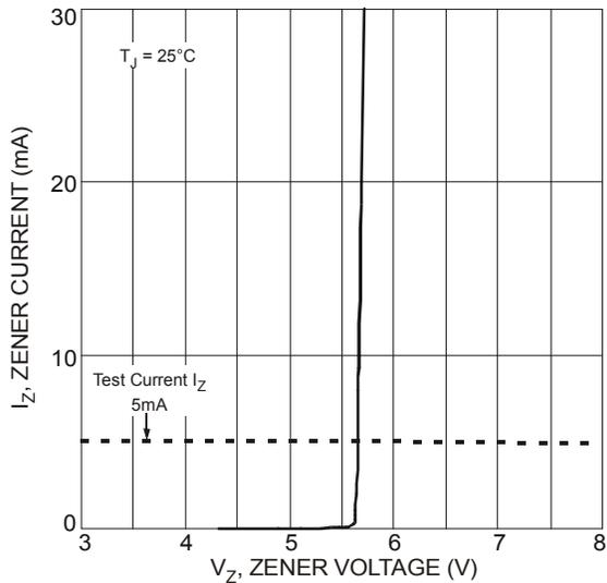
Figure 3 Typical Zener Breakdown Characteristics, Per Element
